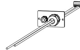
d) Insert the terminal block into the RS485 port of the inverter and tighten the waterproof plug.
