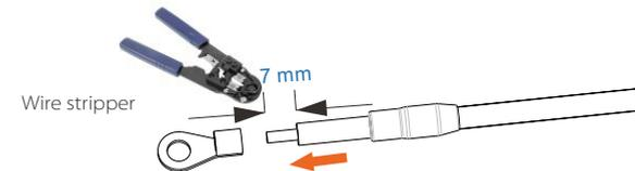
c) Insert the stripped section into the R-type terminal and crimp it.
