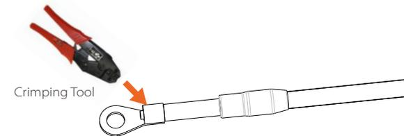
d) Pull the terminal sleeve over the crimped section of the R-type terminal and make sure it is firmly contacted with the terminal.
