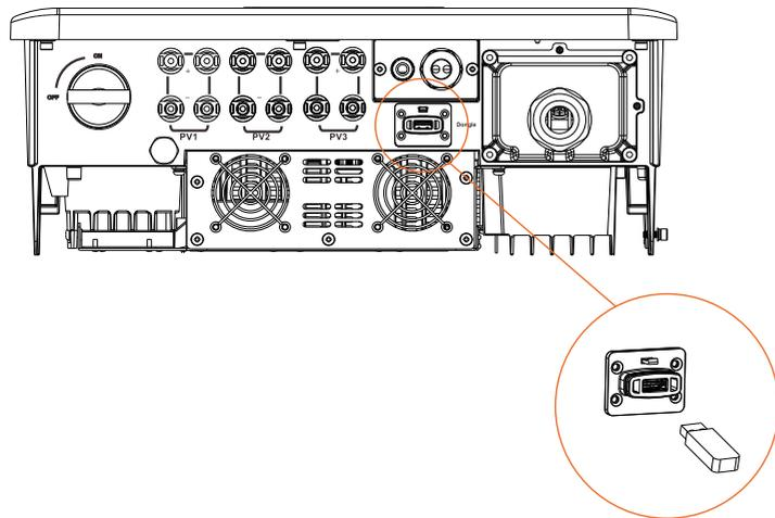
3) Then insert the U-disk into the Dongle port on the bottom of the inverter. Then turn on DC switch and connect the PV connector, the LCD will show a picture as below.
