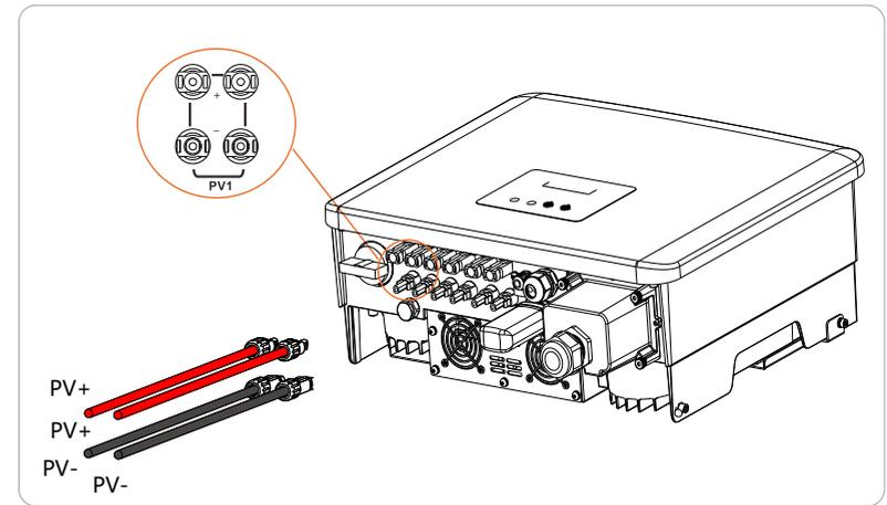
Schematic diagram of the inverter PV connected.
