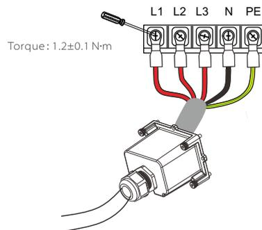
j) Align the waterproof cover and tighten the four screws with an inner hexagonal wrench.
