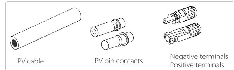
Step 2. Use a wire stripper to strip 7 mm insulation layer from the wire end.
