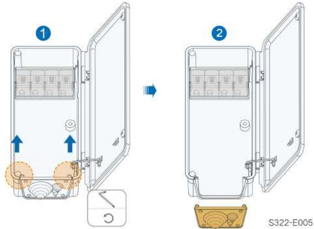
**i** The screws on the sealing plate are captive screws. When the sealing plate is removed, the screws remain on it.
