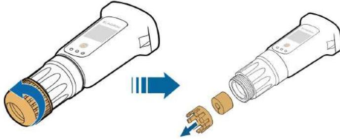
step 3 Unscrew the housing from the communication module.
