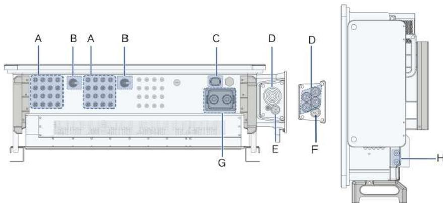
figure 5-2 Terminal Description(SG75CX-P2)
