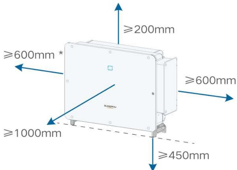
\* In case this distance is less than the distance in the diagram, move the inverter from the mounting-bracket or wall before maintaining fans.
