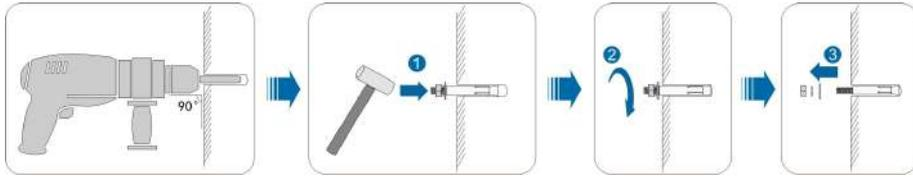
**i** After removing the nut, spring washer, and flat washer, level the front of the expansion tube with the wall. Otherwise, the mounting brackets will not stay steady on the wall.
