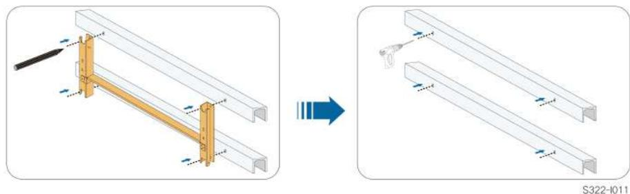
step 3 Secure the mounting-bracket with bolts.
