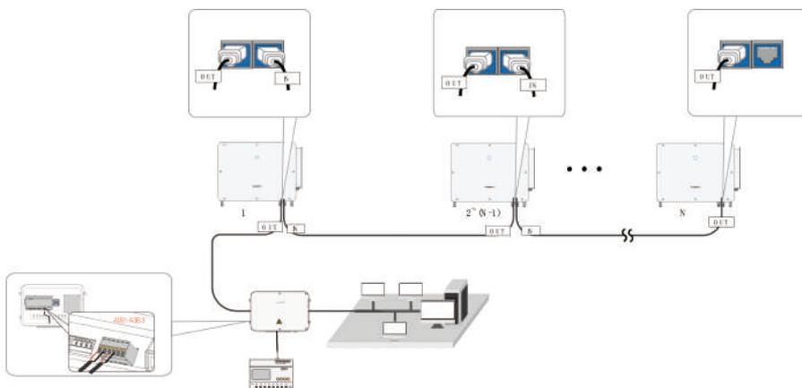
**figure 5-7** Multi-inverter Communication System 【RS485\_1 interface (RJ45)】
