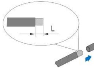
step 2 Assemble the cable ends with the crimping pliers.
