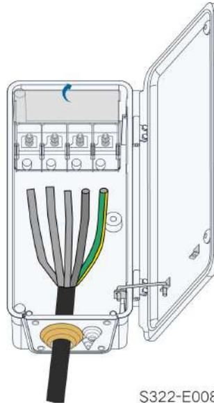
step 7 Connect cables with crimped OT/DT terminals to corresponding terminals and secure them. Please fasten AC terminals referring to the torque specified on the label inside the AC box.
