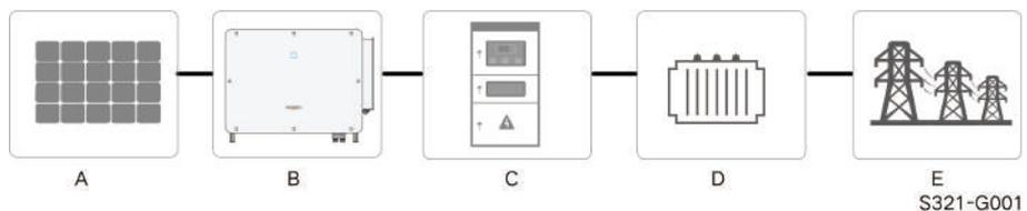
figure 2-1 Inverter Application in PV Power System
