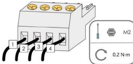
step 6 Insert the terminal socket into the corresponding terminal block.
