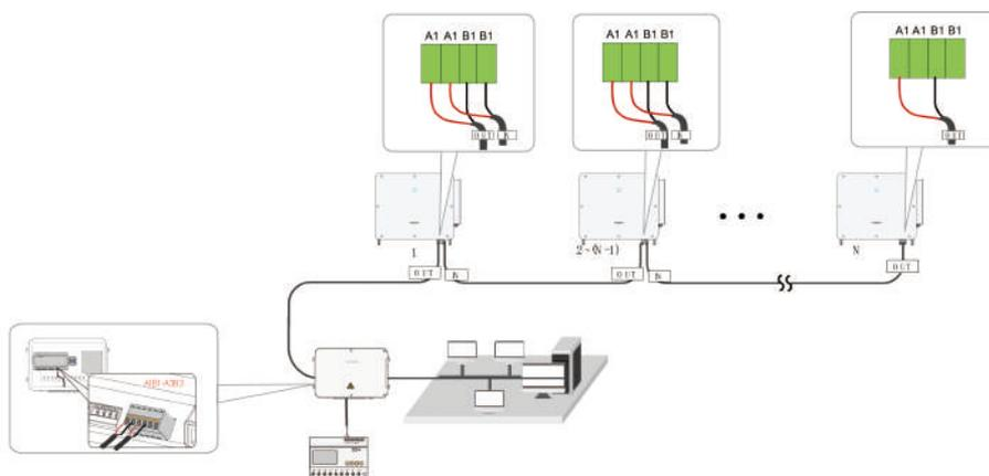
**figure 5-6** Multi-inverter Communication System 【RS485\_1 interface (terminal block)】
