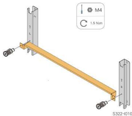
step 2 Level the assembled mounting-bracket by using the level, and mark the positions for drilling holes on the PV bracket. Drill the holes by using an electric drill.
