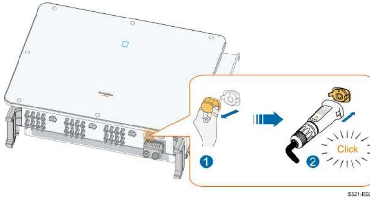
step 7 Slightly shake it by hand to determine whether it is installed firmly.
