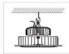
③ Hang the safety rope on the hook
