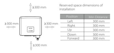
The distance of installation space for multiple inverters is as follows:
