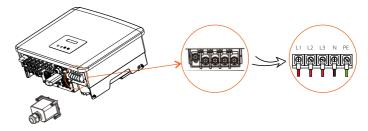
d) Unscrew the fastening nut of the AC waterproof cover and remove the sealing rings. Select appropriate number of the sealing rings according to the outer diameter of the cable. Let the cable pass through the fastening nut, the sealing ring(s) and the waterproof cover in sequence.
