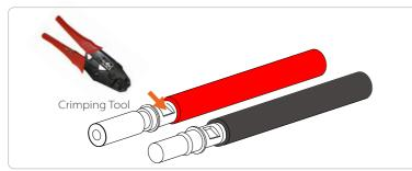
Step 5. Divide the PV terminal into 2 parts - the plug and the fastening head. Insert the cable through the fastening head and the corresponding plug. Note that the red and black lines correspond to different plugs. Finally, force the cable pair into the plug, there will be a "click" sound, which indicates that the connection is completed.
