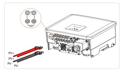
Schematic diagram of the inverter PV connected.
