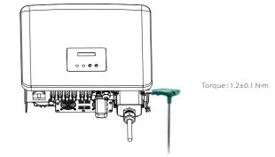
k) Tighten the waterproof fastening head.
