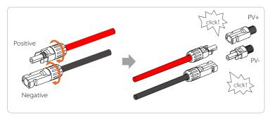
The following is the location of the inverter's positive and negative (PV+/PV-) ports.
