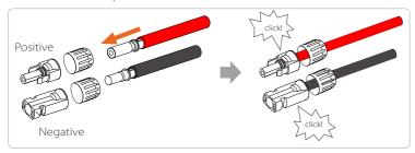
Step 6. Tighten the fastening head and insert into the corresponding positive and negative (PV+/PV-) ports of the inverter.
