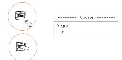
4) Press the "Up" and "Down" button to select ARM or DSP. Then long press "Down" and select the correct update file to confirm the update. ARM and DSP shall be updated one by one.
