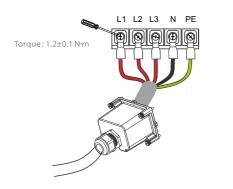
j) Align the waterproof cover and tighten the four screws with an inner hexagonal wrench.
