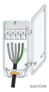
step 7 Connect cables with crimped OT/DT terminals to corresponding terminals and secure them. Please fasten AC terminals referring to the torque specified on the label inside the AC box.
