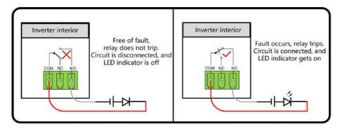
figure 5-8 Normally open contact
