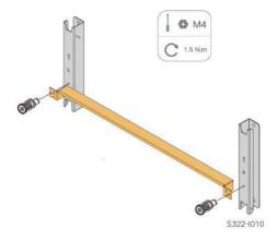
step 2 Level the assembled mounting-bracket by using the level, and mark the positions for drilling holes on the PV bracket. Drill the holes by using a electric drill.
