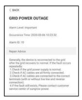
figure 7-9 Detailed Fault Alarm Information
