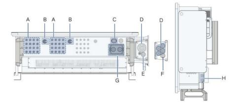
figure 5-2 Terminal Description(SG75CX-P2)
