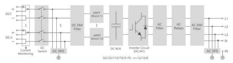
figure 2-4 Circuit Diagram
