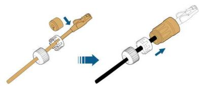
step 5 Insert the RJ45 plug into the front plug connector until there is an audible click and tighten the housing. Install the gasket and fasten the swivel nut.
