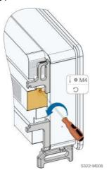
step 3 Press the tab of the latch hook, unplug the cable connection joint outwards, and loosen the screw on the fan holder.
