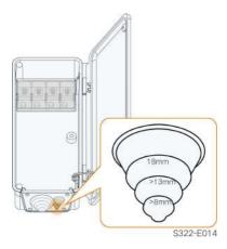
step 3 Lead the cable through the seal ring. The length of unstripped cable in the AC junction box is 50mm.
