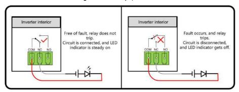
figure 5-9 Normally closed contact
