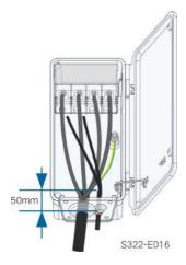
step 4 Place the OT terminals of power cable for tracking system on the OT/DT terminals of the AC cable, and secure them.
