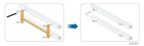
step 3 Secure the mounting-bracket with bolts.
