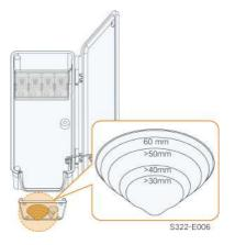
step 5 Lead the cable with the protective layer stripped through the sealing ring and secure screws on the bottom sealing plate.
