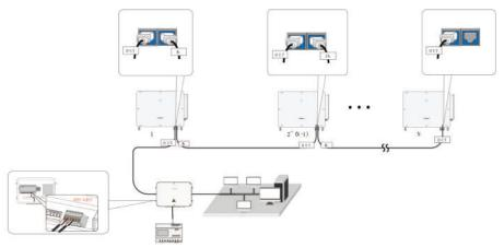
figure 5-7 Multi-inverter Communication System 【RS485 1 interface (RJ45)】
