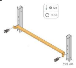
step 3 Mark and punch holes in the U-beam according to the dimensions shown below.
