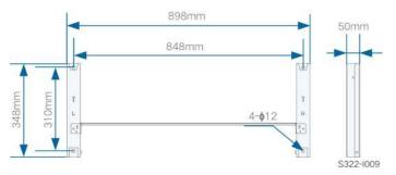
figure 4-1 Dimensions of Mounting-bracket
