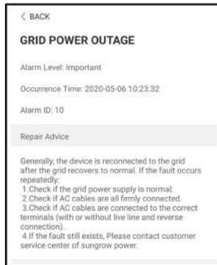
figure 7-8 Detailed Fault Alarm Information
