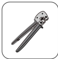
OT terminal crimping tool (4 mm 2 –6 mm 2 )
